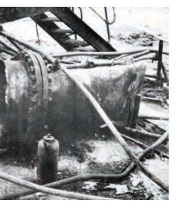
exposed orifice, but the jacknifed pipe still attached at its other end (insufficient force to eject it), the explosion would have occurred. That, he says, would account for the evidence of burning in a carburising atmosphere at one bellows end, but not the other. Now the blast would tear off the Reactor Six end and propel it to the ground, hitting Reactor Six on the way (damage possibly attributable to that event was photographed) and impacting with the concrete reactor plinth below (ditto).
